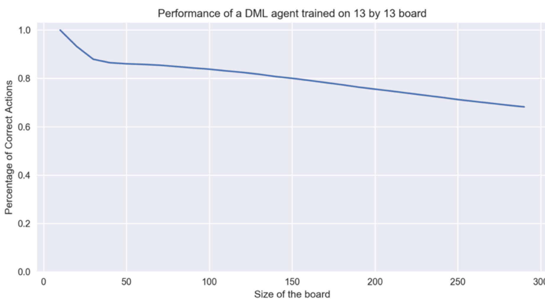
Figure 6. Performance of a Model Network that the DML agent converged to through datasets received from a Q-Network trained on a 13 by 13 board. Single layer feedforward network with cross-entropy cost function, trained for 2000 epochs.
