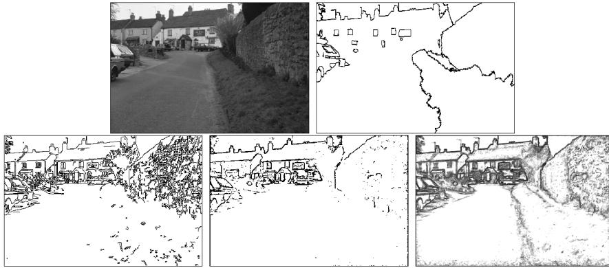
Fig. 1. A typical Sowerby image (top left panel) with its ground truth segmentation (top right panel), and its segmentation using the Canny edge detector (bottom left panel) and by statistical edge detection (bottom center panel). Statistical edge detection has fewer false negatives in the textured regions and is also better at detecting edges with are partially defined by texture. By contrast, the Canny detector is slightly better at precision of certain edges. The log-likelihood ratios are also shown (bottom right panel).
