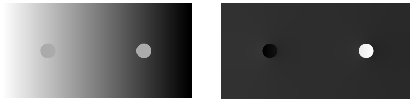
Fig. 5. Simultaneous contrast illusion. Left: the original image. Right: Retinex result with t = 3 . By Retinex the background slope is eliminated and therefore the shape-background contrast enhanced. In the left image the two disks have exactly the same grey level. Retinex is an attempt to formalize the process by which the right disk appears conspicuously brighter than the left one. After applying Retinex, this disk indeed becomes brighter.
