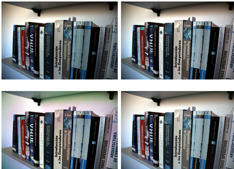
Fig. 8. Top Left: Original image. Top Right: Retinex result applied to the raw image with t = 0 . Bottom Left: Retinex result with t = 0.05 . Bottom Right: Retinex result applied to the gamma corrected image with t = 2 . Notice how similar are the results. Both maintain an image that is close to the original, but the low contrasted texture on the wall has been wiped out.
