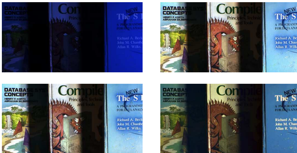
Fig. 12. Top Left: Original image, Top Right: Result of McCann99 with 4 iterations, Bottom Left: Result of Frankle-McCann with 4 iterations, Bottom Right: Result of PDE Retinex.
